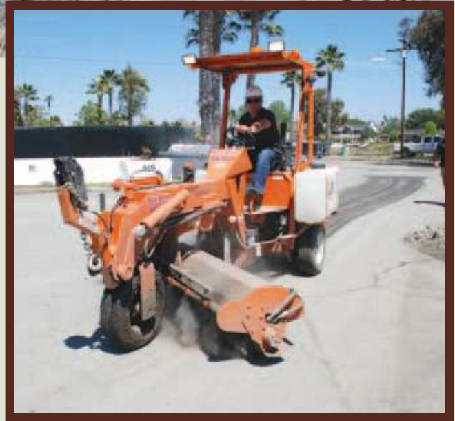
(Above Left) Cat wheel loader rented from Heavy Equipment Rentals moves and loads filtered silt, sand and dirt onto end-dumps for transport to the Port of Long Beach to be used as fill material. (Above Right) Sweeper rented from HER keeping dirt and dust levels down to a minimum.
